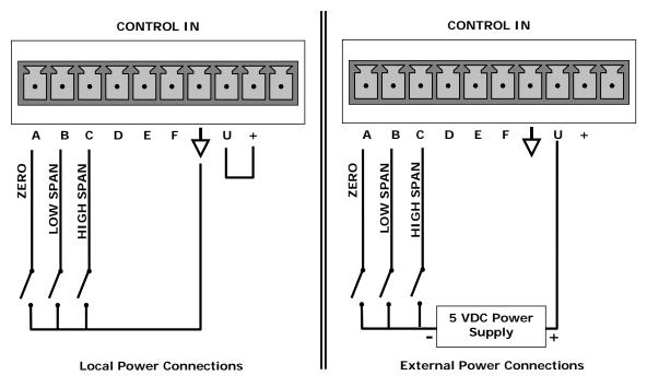
Figure 3-12: Control Input Connector
